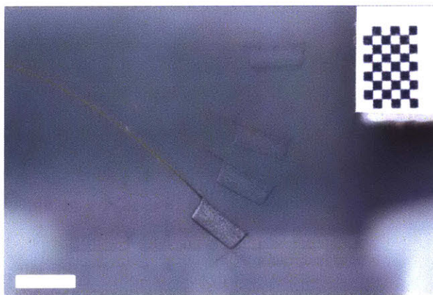
Figure 4.2: Sample overlay of photographs used for cantilever deflection measurement. Scale bar is 3 mm.
