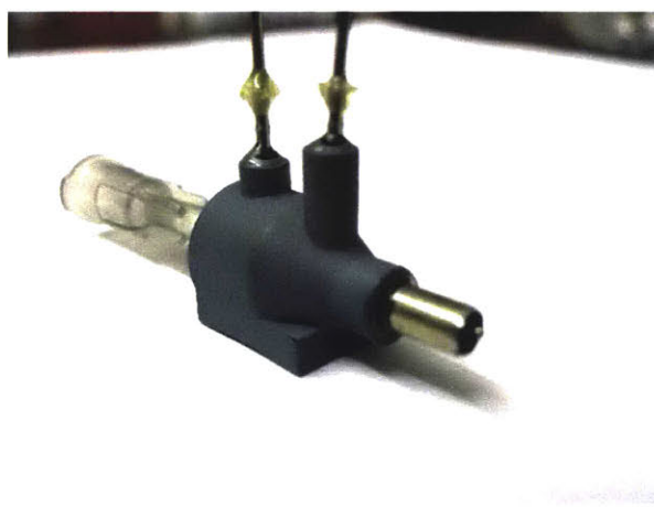
Fig. 2. The 3D-printed nozzle assembled with needles.
