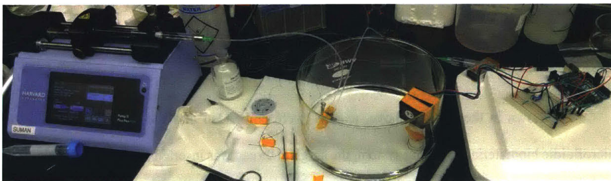
Fig. 3. Assembly of alginate-thread depositing system. From left to right: syringe pump, nozzle at base of dish, motor with spool attached to side of dish, breadboard with Arduino chip and LED for spool speed display.
