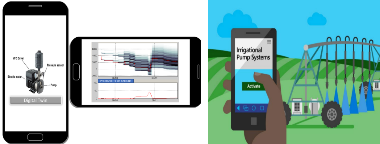
Fig 2: Monitoring mean time between failure (MTBF) from sensor data on a mobile smartphone (L). With decreasing residual lifecycle (upper panel) the probability of failure (broken part may precipitate unplanned downtime) increases (lower panel). Just in time spare parts supply chain coordination with maintenance, using MTBF data, prevents potential machine failure. Probability of failure drops to “zero” (lower panel) when the part at risk is
