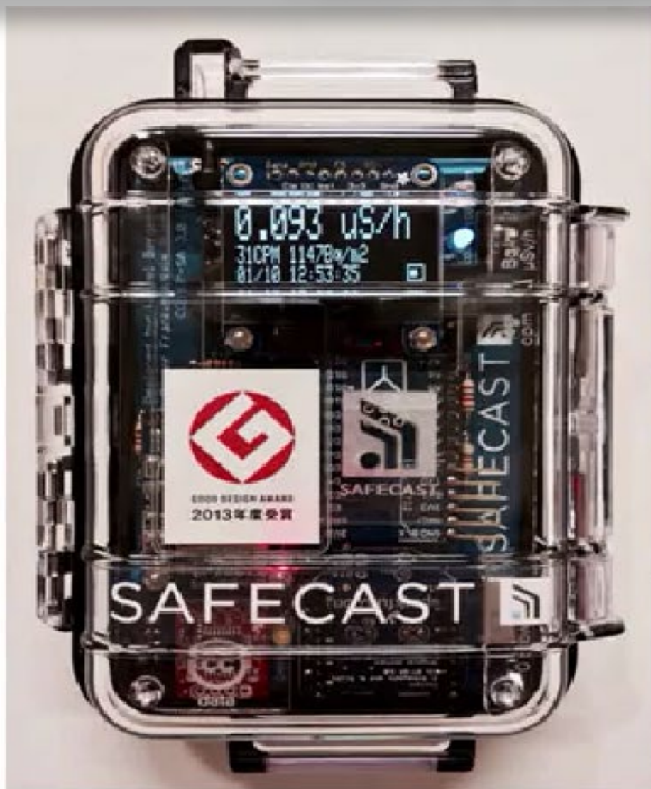
Safecast Nano - Mobile Radiation Monitoring Wireless Geiger Counter, GPS with Bluetooth
