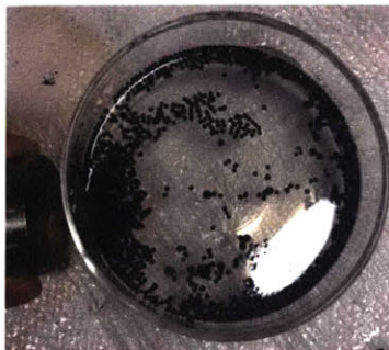
Figure 3-2. Magnetic response of the organo-alginate hydrogel
