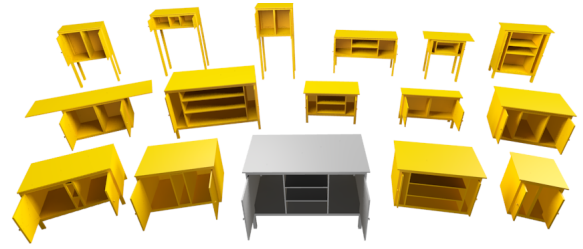
Figure 3: An example of a template. The original design is shown in gray, and new designs generated by varying the template parameters are shown in yellow.
