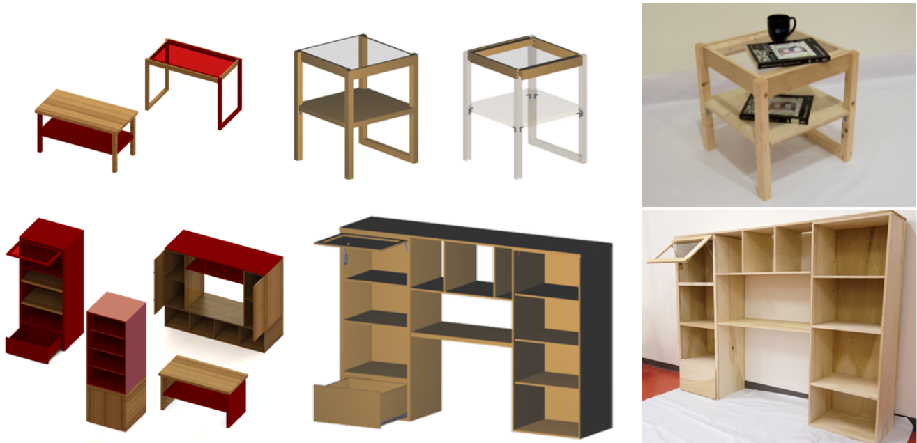
Figure 13: From left to right: input designs, models created using the system, and fabricated results. We highlight the connecting elements on the first model by making all principal elements semi-transparent.
