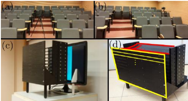
Figure 16: Our prototype and capture setup. (a) The auditorium in which images were captured. A camera was placed on a rod and was moved horizontally to simulate the movement of a viewer's head. (b) Capturing was performed at several seats in the auditorium. (c) The barriers assembly and the LCD screen behind it. (d) Emphasizing the vertical barrier (yellow) and the horizontal slanted barrier (red).
