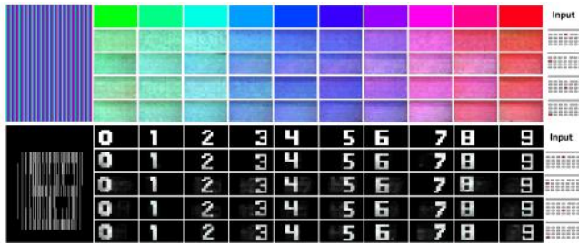
Figure 15: Two test scenes illustrating the angular resolution of the display. Top row: 10 target patterns used as angular images. Rows 2-5: the patterns captured from different rows and seats, illustrating accurate reproduction of the target. Left: The interlaced angular images as displayed on the back screen. Right: the seat at which this row of angular images was captured, marked over the auditorium layout.
