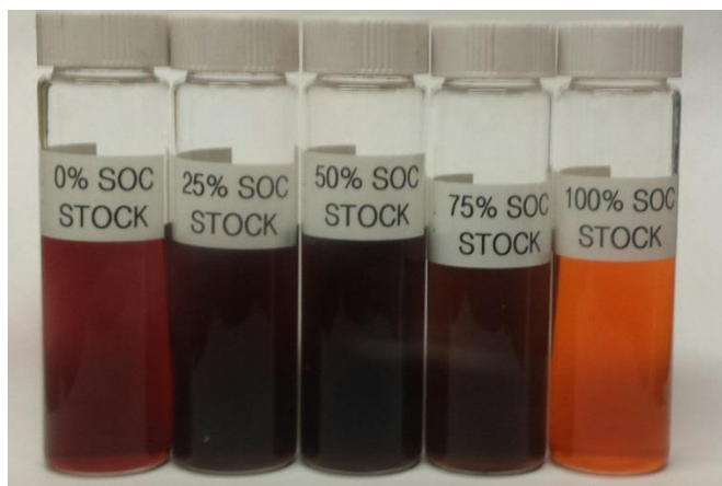
Figure 4: 0.5 M AcNH-TEMPO solutions in 1 M LiBF 4 / PC at 5 SOC (0 %, 25 %, 50 %, 75 %, and 100 %).
