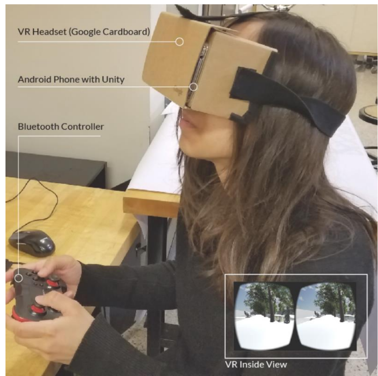
Figure 5: VR Review Experiment Setup with Google Cardboard and Bluetooth Controller
