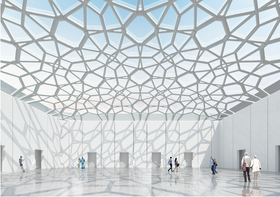
Figure 5-1: Concept rendering of a grid shell roof structure designed in phase two, where the force densities are scaled. The variables used to generate the form are as follows: d = 5 , o_1 = 1.0 , o_2 = 1.0 , and h_{target} = 1 . Rendering produced by Daniel Marshall, MIT.
