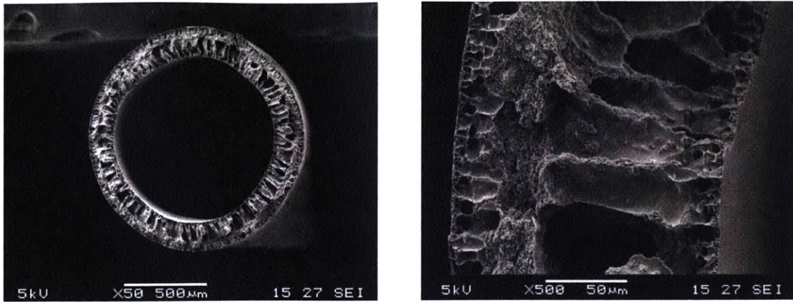
Figure 2-1: From Wang et al. [2009]. Typical cross-sectional microstructure of a PVdF porous fiber membrane.
