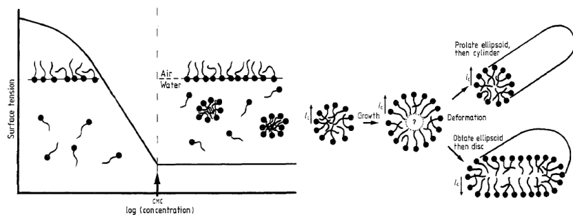
Figure 1.8. Schematic of micellization processes (Reference 35).
