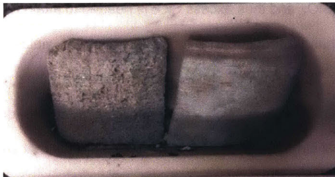
Figure 15: Balsa and pine specimens soaked at a lower concentration did not collapse and disintegrate after firing.
