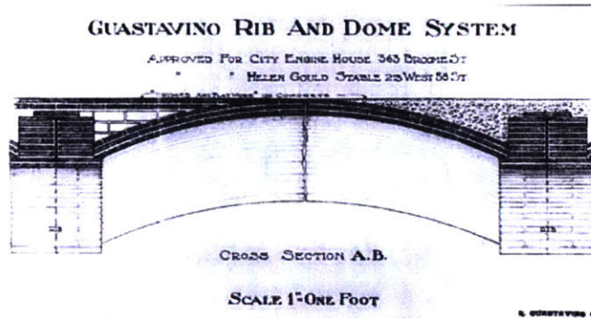
Figure 6.4: Guastavino Rib and Dome System (ca. 1902, New York; Guastavino/Collins Collection, 1902)
