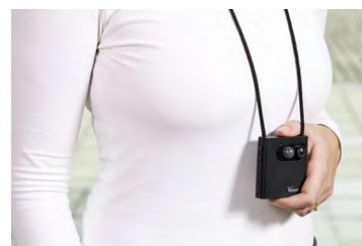
Figure 9: Microsoft SenseCam, a wearable life-logging device. Credit: Microsoft.
