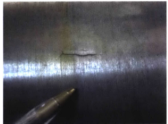
Figure 11: (a) Magnetic Particle Inspection Methodology for R2R Substrates [24] (b) Crack Identification due to Selective Binding of Magnetic Particles [25]
