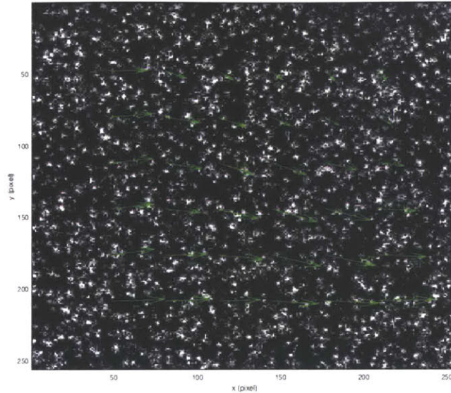
Figure 4.5: Mpiv result. Green arrows represent the swimming direction of the bacteria. The longer the arrow, the faster the swimming speed is.
