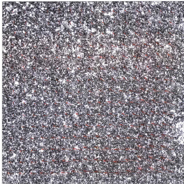
Figure 6.4: PIVlab analysis result of original image pair, interrogation window 256 pixels, with 50% overlapping. Before PIVlab running, the contrast of the images is firstly enhanced by “adapthisteq” command and the threshold are changed to 30,000.
