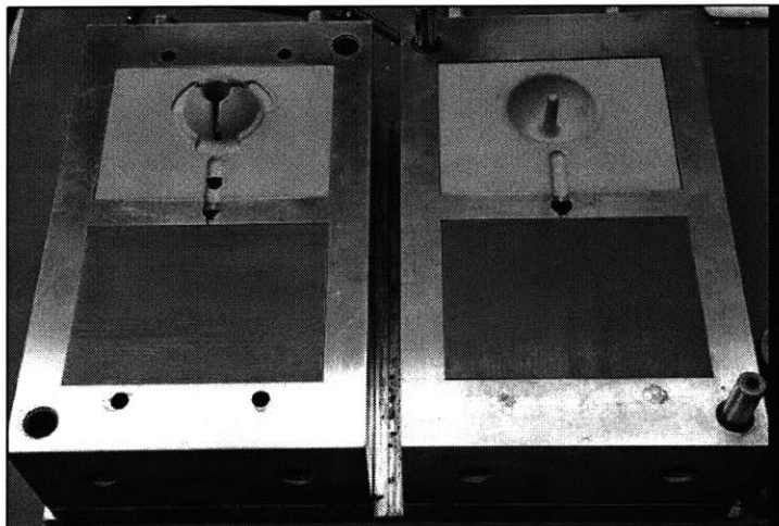
Figure 43: Experimental setup with metal-polymer blend injection-mold inserts
