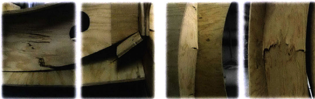
Fig. 5.20 Failure Modes – GEN.2_Initialized: Details (a.) Invert; (b.) Axial.
