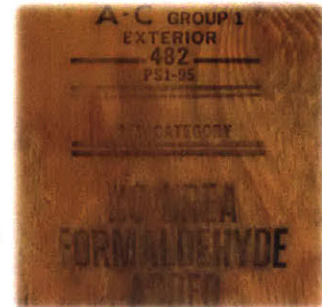
Fig. B.2 BOD – Plywood: Group 1. Only veneer grades: N, A, and C.
