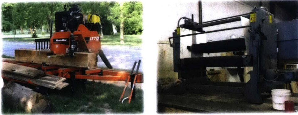
Fig. 1.7 Conventional Construction – Pre-process is constraining: (a.) Portable sawmill; (b.) Industrial laminator.
