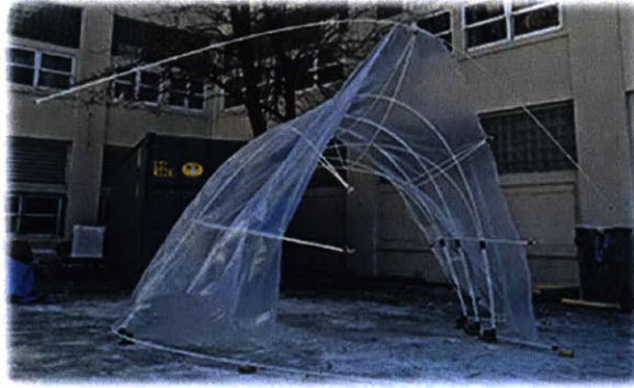
Fig. 7.3 Contributions – Structural: Active bending.
