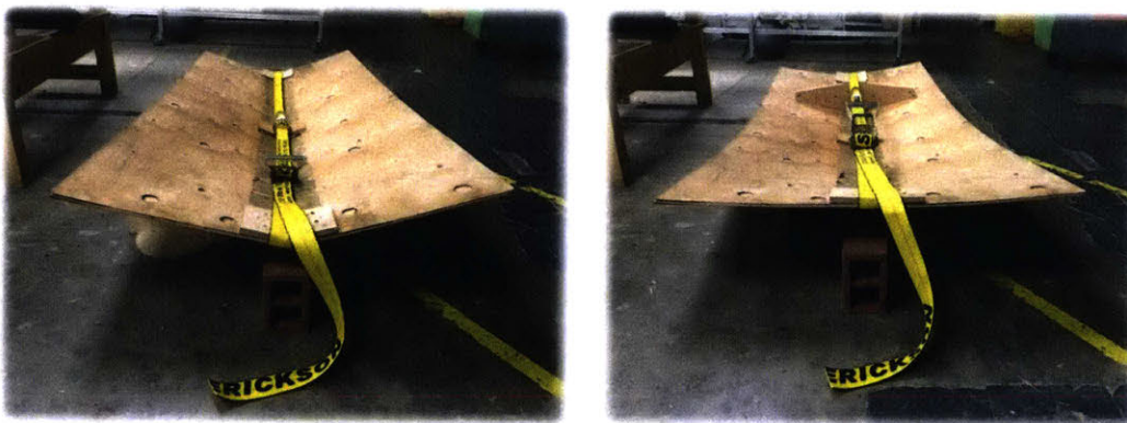
Fig. 4.20 Mockups – GEN.3_Hinges, Method: (a.) Strips only; (b.) Strips with Wedge.
