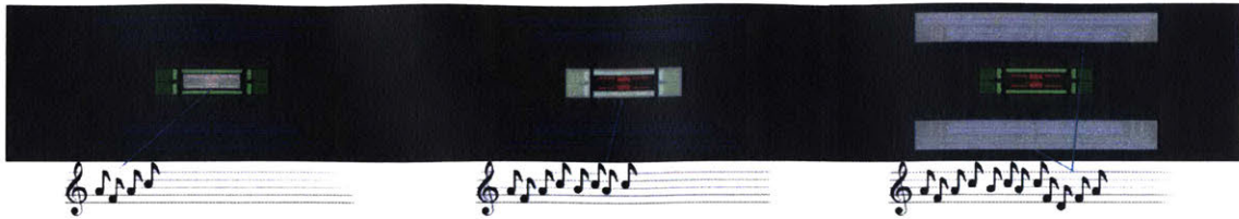
Figure 2-5: Data streaming order when the composer sets the Python ‘spatialized’ flag to ‘true’. First, inner detector data is streamed, followed by calorimeter data. Lastly, RPC data is streamed. Each individual layer is streamed with respect to the layer’s theta coordinate. Alternative streaming modes are supported as well.
