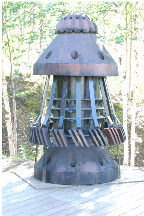
Figure 1-3: A cleaning pig used on the Trans-Alaskan Pipeline[10]
