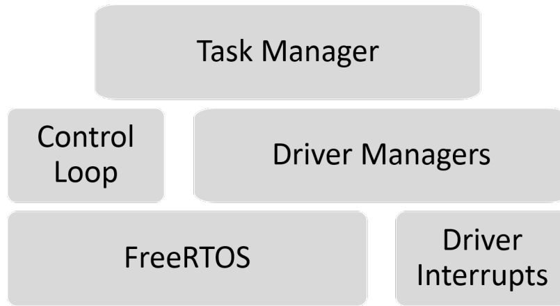
Figure 4-1: The Task Manager is responsible for the most abstract forms of control, and it sends commands to the middle layer managers. These direct the hardware in synchronous tasks, and set up driver interrupts to handle asynchronous tasks.
