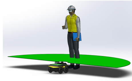
(b) Lidar at shin height
