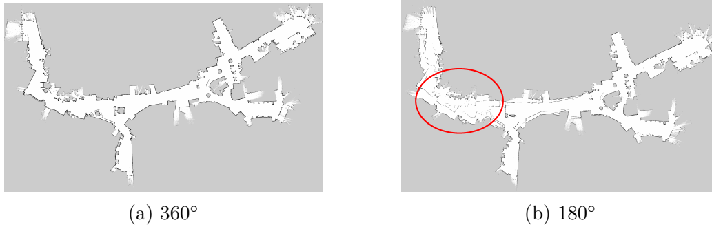
Figure 4-6: Maps Generated with Full and Limited Angular FOV (Velodyne)
