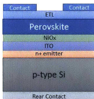
Figure 5: Perovskite-Si 2T tandem device with generic p -type Si bottom subcell.
