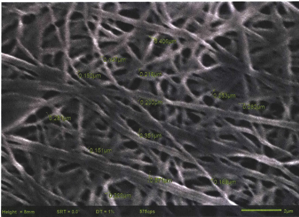
Figure 151: fiber diameter after pressing
