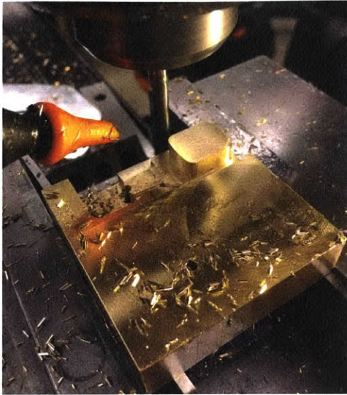
Figure 104: Fabrication of the matching sliders
