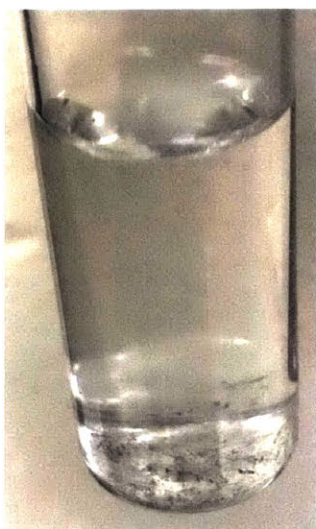
Figure 164: pill dissolves in water & metal contamination residues stay visible
