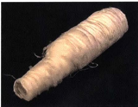
Figure 147: the stripped polymer before pressing
