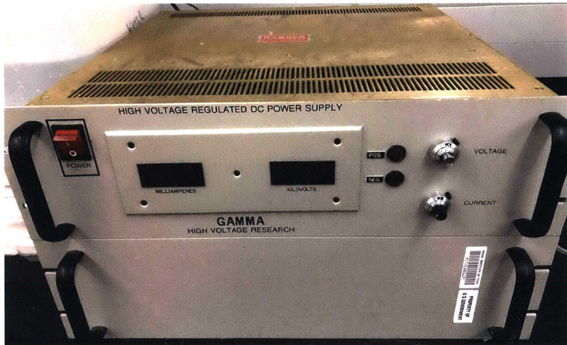
Figure 79: High Voltage Power Supply for Electrospinning
