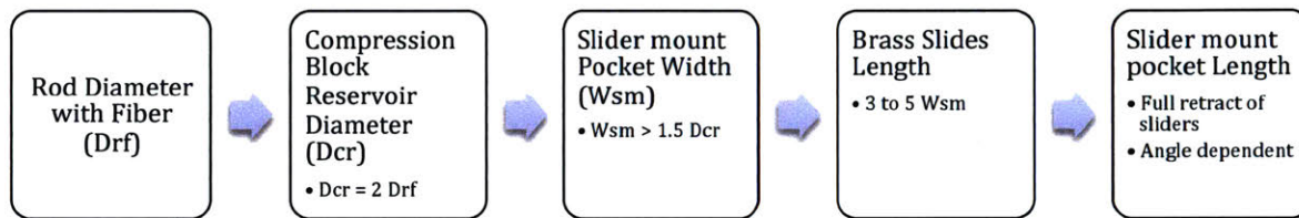
Figure 102 Process for specifying geometry of components
