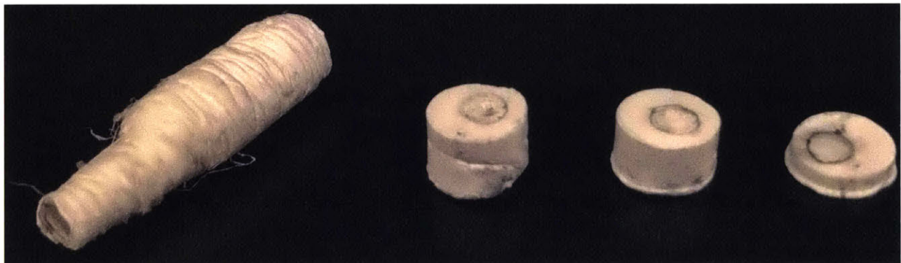
Figure 171: un-pressed mix and pills pressed at different pressures
