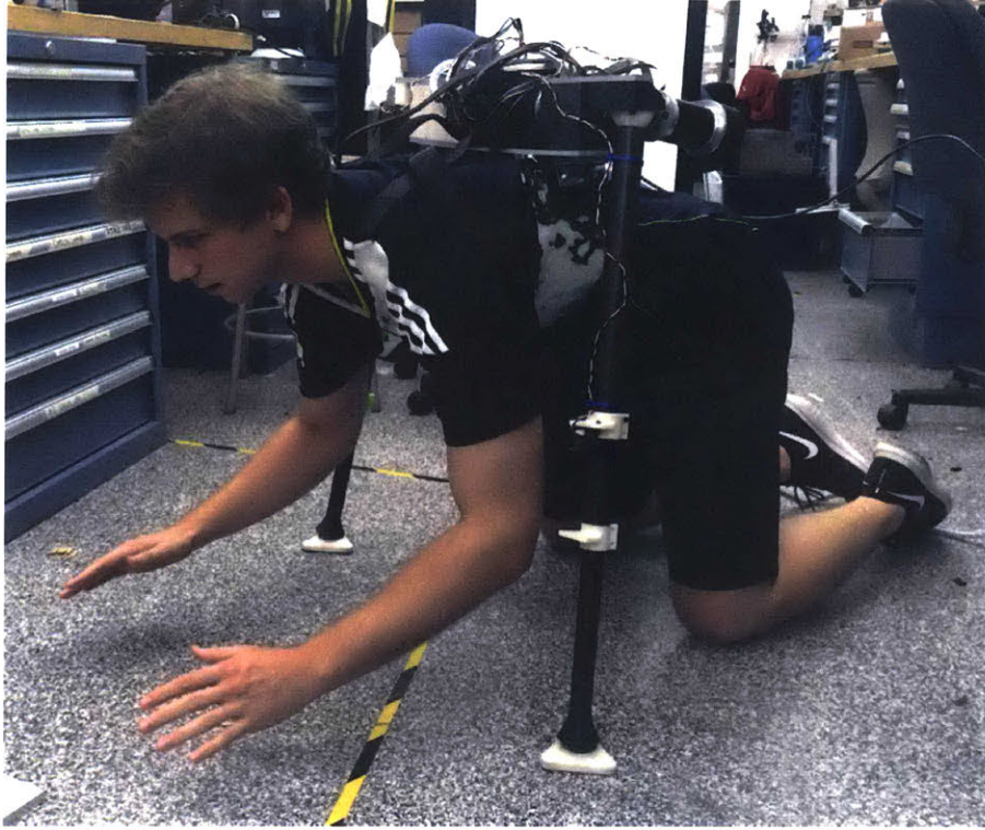
Figure 3-1: Prototype of the MantisBot used to test impedance control law.
