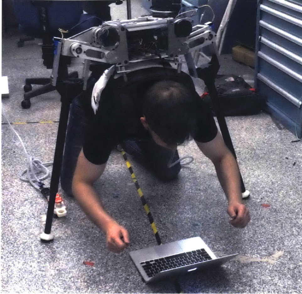
Figure 3-3: Second prototype in operation with static legs
