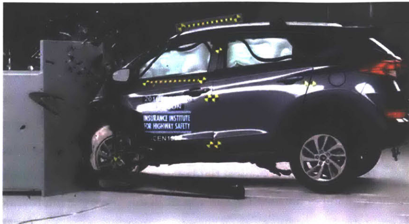
Figure 1-3. Small overlap crash test of 2016 Hyundai Tucson (courtesy of the Insurance Institute for Highway Safety)
