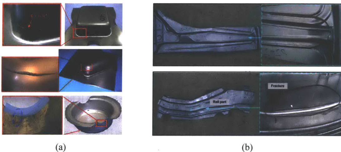
Figure 1-2. Ductile fracture during sheet metal forming: (a) square and circular cup drawings of TRIP690 steel (Li et al., 2010) and (b) B-pillar stamping of DP600 and DP980 steels (Sung, 2010).
