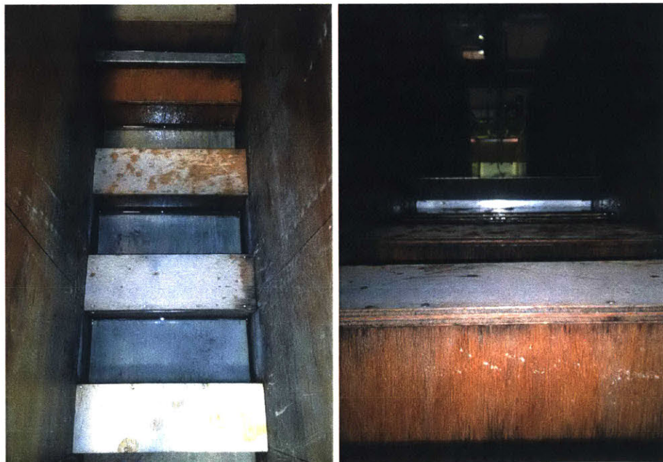
Fig. 2.19. A wind catcher prototype fixed to the sidewalls above the fourth model block. Left: top view where the flow direction is from the bottom to the top, right: view from the flow direction.
