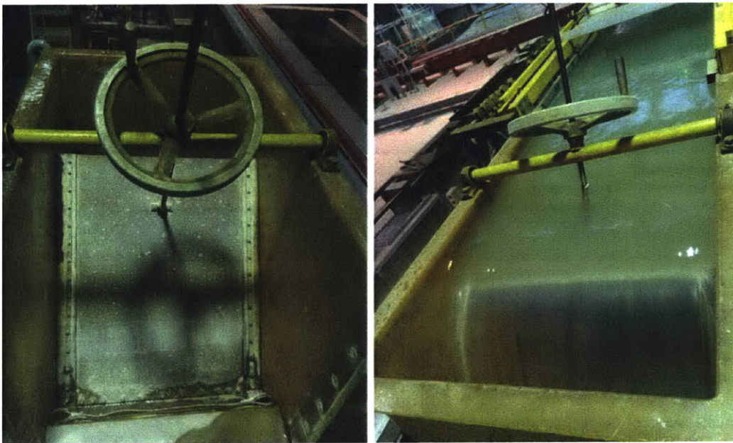
Fig. 2.3. Adjustable floodgate to vary water depth. Left: viewed from upstream of the floodgate (no water), right: viewed from the end of the channel with water flowing.
