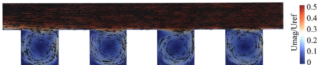
Fig. 3.4. Normalized velocity magnitude contours and vectors in canyons 3, 4, 5 and 6. All canyons have identical flow field with a large clockwise-rotating vortex.
