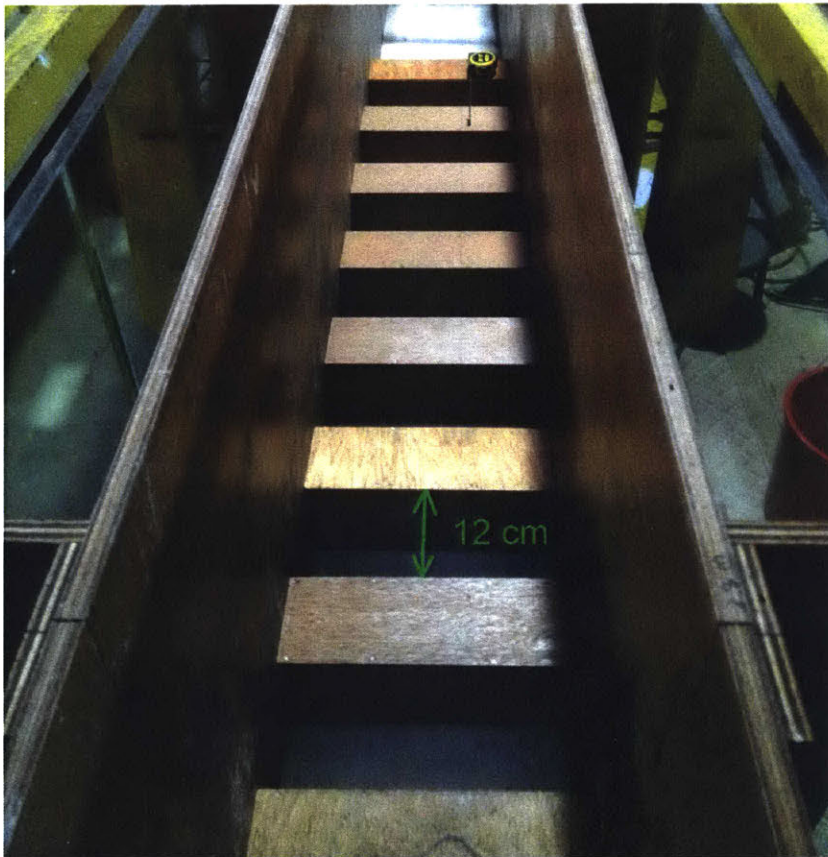
Fig. 2.11. Arrangement of seven 12 cm tall \times 12 cm wide canyons with aspect ratio 1 in the test section.
