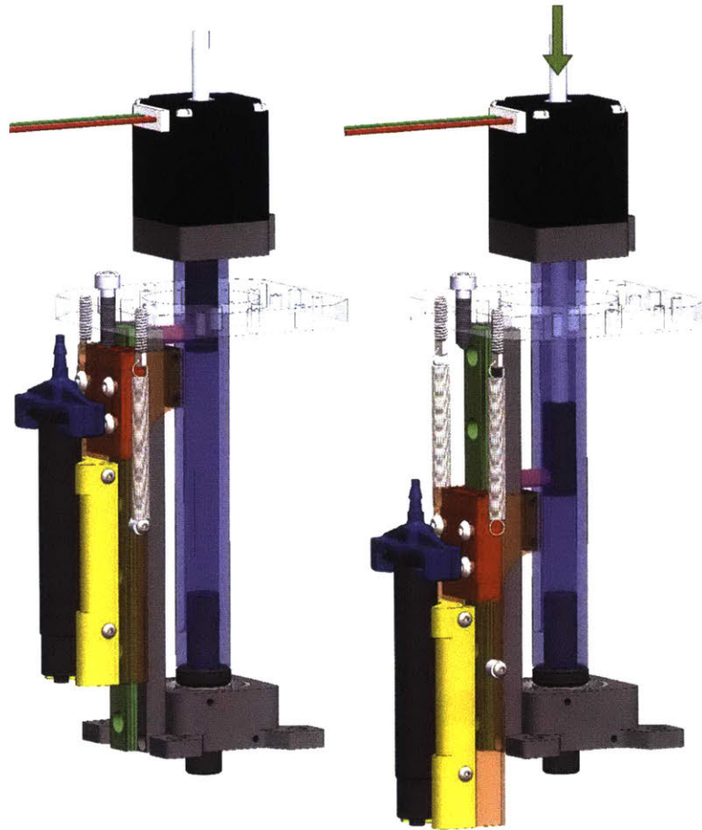
Figure 4.5: Cross section of carousel assembly in raised state (left) and lowered state (right). The position of the non-captive stepper motor shaft and slider block with drive pin (pink) can be seen inside of the drive tube (transparent blue). Also shown are the bearing block (red), linear rail (green) and the counterbalance springs. Only one syringe rail assembly shown for clarity.
