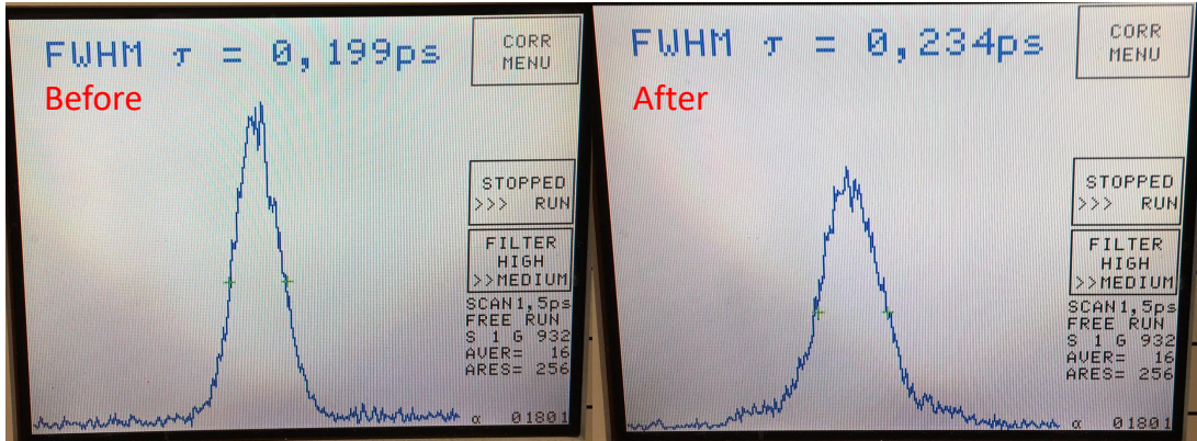
Figure 4-2: 6.25-nm pump autocorrelation measurements before and after the spectral filter system. The left figure shows the pump pulse duration before the spectral filter system and the right figure shows the pump pulse duration after the spectral filter system. A factor of 1/\sqrt{2} exists between the real pulse width and the measured quantity.
