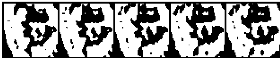
Figure 4-7: Five adjacent slices sampled from the X-ray tomography data used for the 3D compression experiment. Note the strong continuity in the third dimension.
