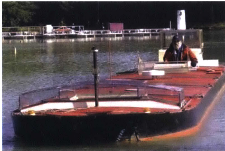
Figure 6: Scale Model For Training Cargo Captains (Scale 1/25)
