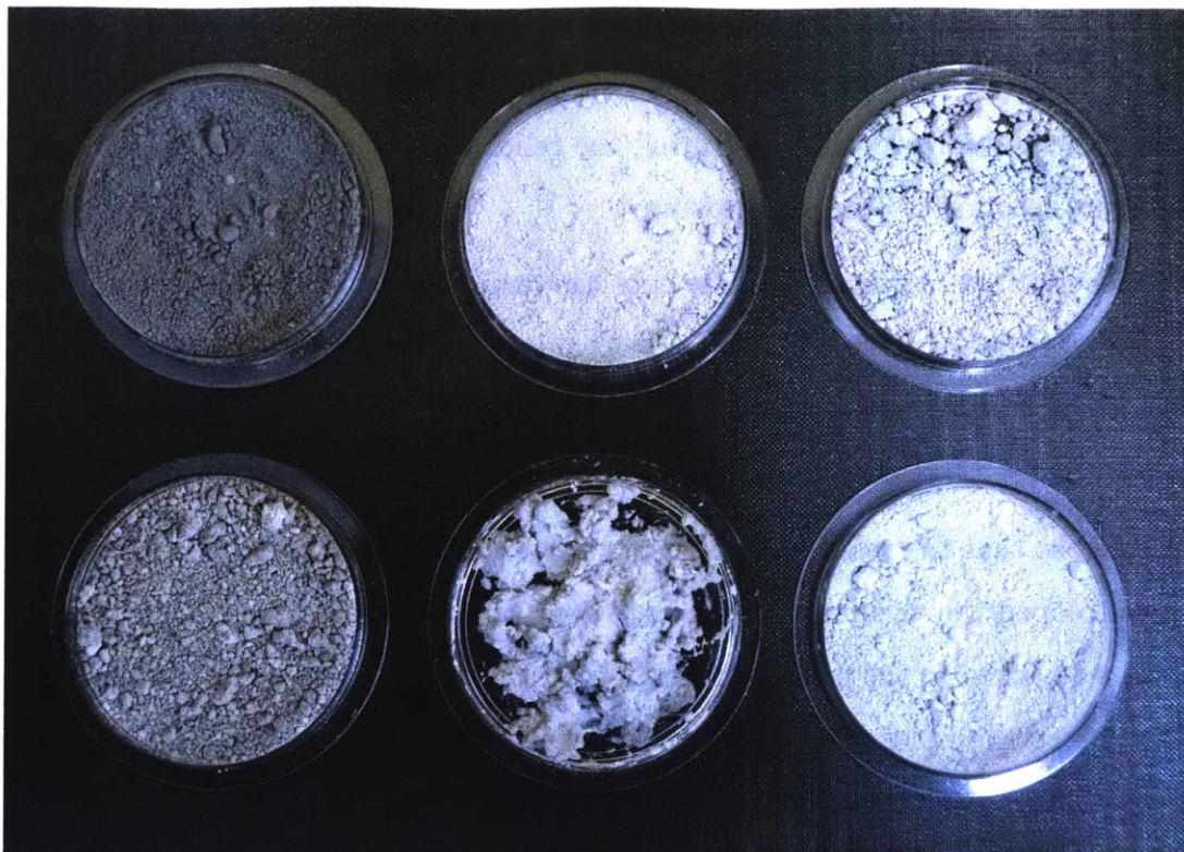
Figure 3-7: Images of oxidized aluminum byproducts from testing. Top row, left to right: atmospheric pressure, 1035kPa, 1725kPa. Bottom Row, left to right: 3450kPa, 5170kPa, 6900kPa
