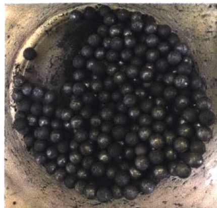
Figure 1-5: Aluminum fuel treated with gallium/indium eutectic through Slocum process [22]
