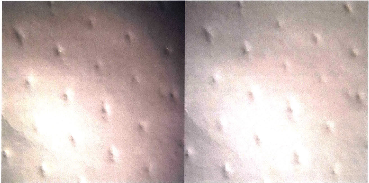
Figure 4-13: Media indentations observed on the location #3 samples and subjecting the substrate to Test B markers.
