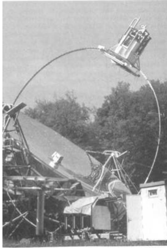
Figure 11: Setup of DCAR with parabolic dish in CAESAR Project [52]
