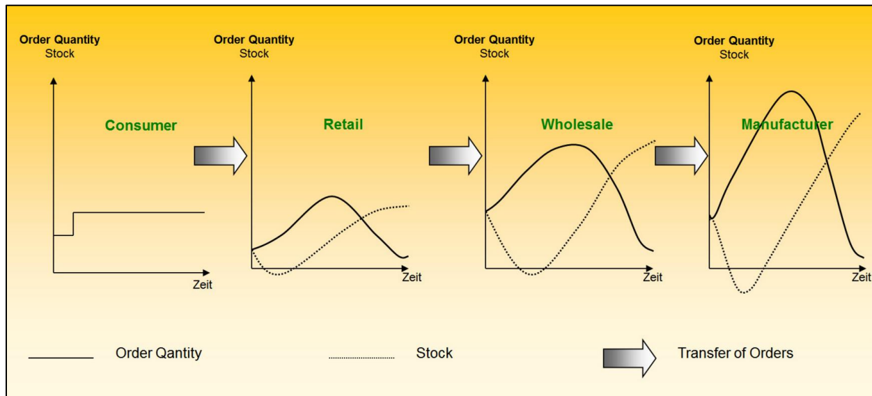
Figure 12: Example of a bull whip effect from point of sale to manufacturer
