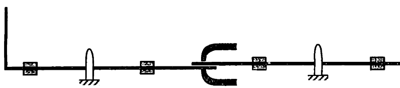
Figure 6.7 Product design alternative: assembly with a lap joint
