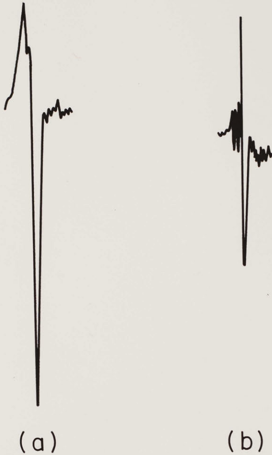
Fig. 12. Auger carbon peak. (a) before sputter etching (b) during sputter etching.
