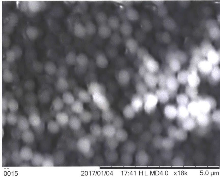
Figure 3-5: SEM of 750 nm SiO 2 beads sintered at 1250 °C. Lighter beads are closer to the electron detector and illustrate the lack of bead packing, which resulted in small chunks sintering together instead of a single sintered mass.
