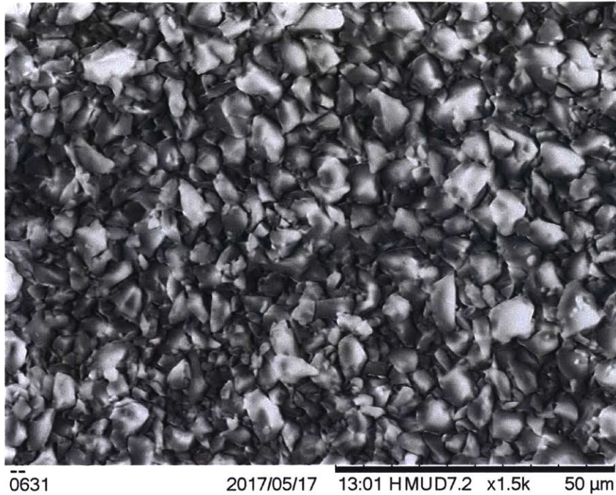
Figure 3-1: SEM of a borosilicate chip used to fabricate emitters. Note the irregularity in particle size and the resulting surface roughness and pore size variation.
