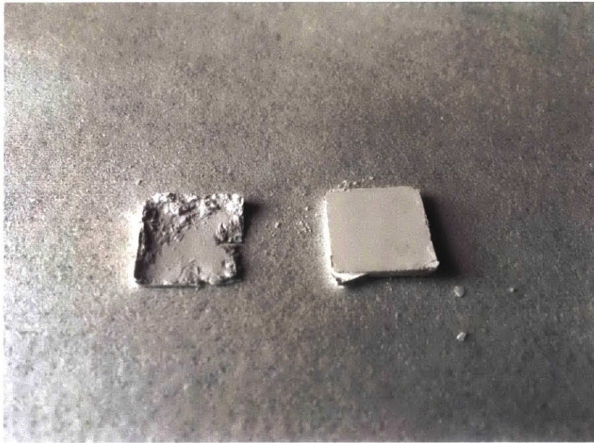
Figure 3-11: Planar layering in a chip after leaving the chip in the hydraulic press for 10 minutes. It was observed that layering occurred more frequently if the chips were left under pressure for durations greater than 20-30 seconds.
