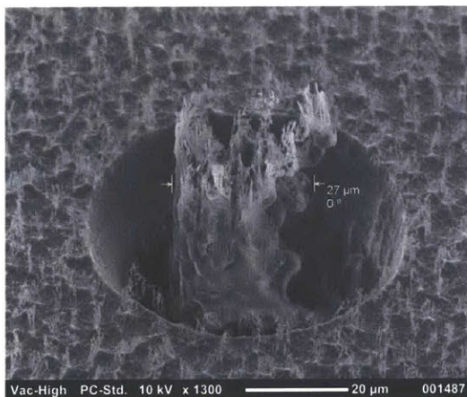
Figure 2-7: RF etched by RIE plasma.
