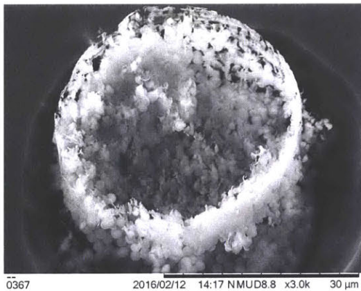
Figure 2-10: SiO 2 micro-spheres coated and bound using soda-lime nano-spheres. If SiO 2 was not fully covered by soda-lime, it was etched away.
