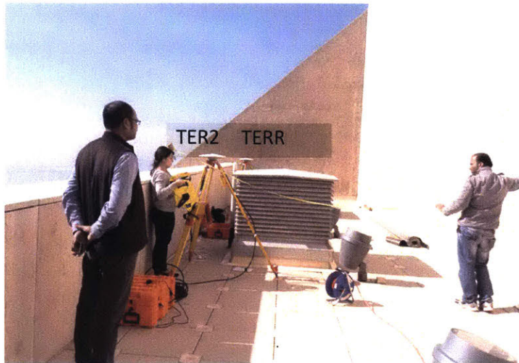
Figure 3.2.2. Al-Hamra terrace GPS sites (TER2 and TERR) located at different distances from the western wall to investigate the effects of multipath. Photos by Thomas Herring .
