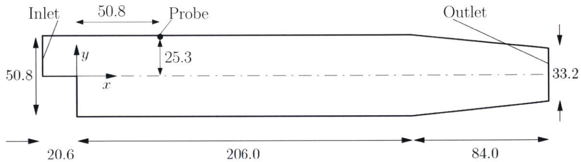
Figure 4-3: Geometry used in the simulation of a chaotic flow over a backward-facing step, dimensions in mm. All boundaries except inlet/outlet are solid walls.
