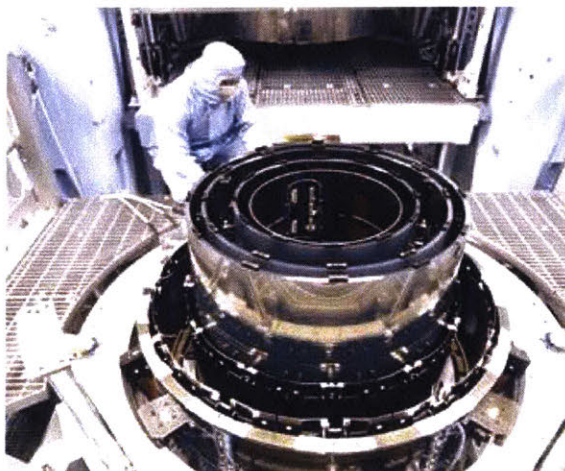
(a) Chandra, launched in 2009, has thick shells ( \sim 25\text{ mm} ) with high resolution ( \sim 0.5\text{ arcsecond} HPD) and small collecting area ( \sim 0.01\text{ m}^2 ). [25]
