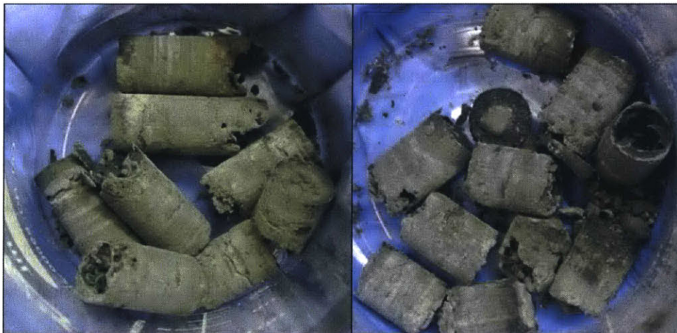
Figure 5-11: Further refinement and more careful design of this batch process is needed. During one test, the piston head rested lower inside the reaction chamber than was intended. This reduced the temperature of the piston head and the adjacent reactants, resulting in incomplete decomposition (right).
