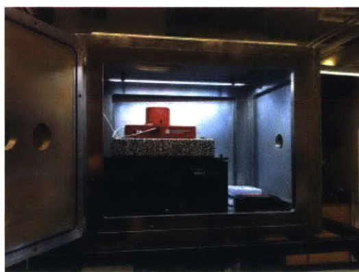
Figure 5.6: The initial test fit of the ezAFM in the vacuum chamber after thorough cleaning and inspection. The AFM (red) is sitting on top of a masonry slab and vibration reducer (black).
