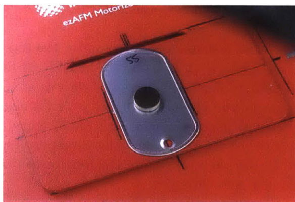
Figure 5.12: A test sample mounted on an SS304 coupon was placed on the stage where it was lightly held by the stage magnets. Tests were run to verify a rough centering alignment could be performed using a glove and a handheld mirror. The stage center would be moved for a more precise positioning.
