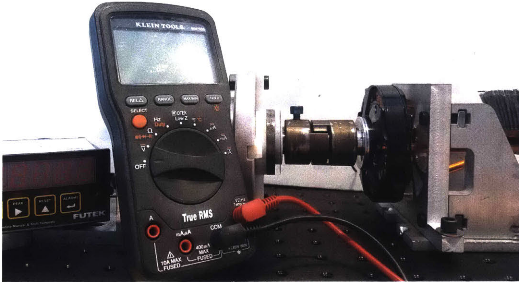
Figure 4-3: Image of experimental setup. Components from left to right: torque readout, voltage readout, torque sensor coupled to motor shaft, motor containing heatpipe insert, heat exchanger.
