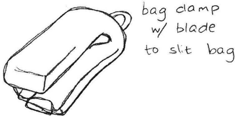
Figure 5: Sketch of stapler-shaped bag clamp idea. Similar to the Easy Glide Bag Opener, this concept would include a blade that would slit a bag open when the clamp is pressed together. This design, however, would be larger so that the clamp could be pressed together simply by exerting one's body weight on it.
