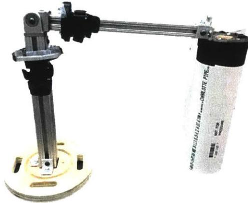
**Figure 1a.** Model leg. The skeleton of the leg is composed of 80/20 aluminum stock. A hinge joint acts as a knee and limits the degrees of freedom available to the leg to one. The black rings shown on the skeleton serve to hold IMUs, which are used to collect data about internal kinematics of the leg. The PVC pipes displayed on the right act as the housing and provide the surface where pressure interactions between the suit and the leg occur.
