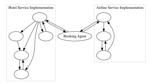
Figure 1-1: An example of a system with logically separate components: a booking agent communicating with a hotel service implementation and an airline service implementation. The booking agent acts as a transaction coordinator to atomically book tickets for both services.
