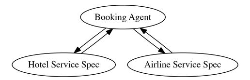
Figure 1-2: The booking agent system building on specifications of the hotel service and the airline service, demonstrating an implementation depending on multiple specifications.
