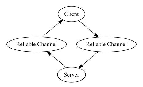
Figure 5-9: Client-server key-value store implementation over reliable channels.
