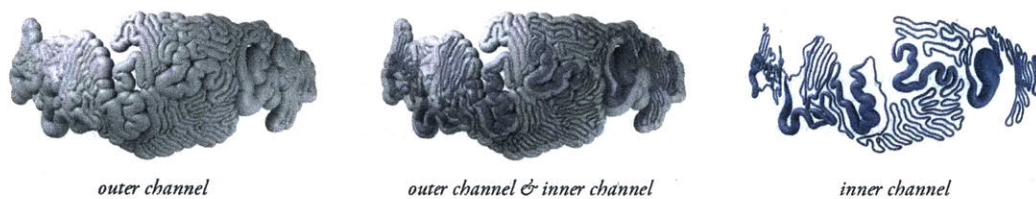
Figure 55 – Visualization of smaller scale test-piece used. The image on the left shows the actual shape of the printed piece. The image in the middle and on the right visualizes how the support material (blue) is distributed and printed inside the wearable to achieve a hollow channel.
