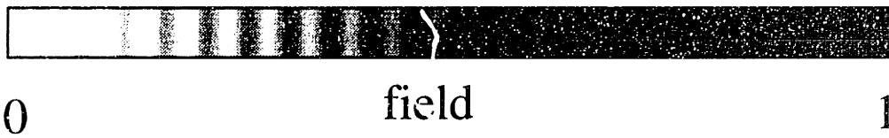
Figure B-1: Electric field at z = 0 \mu\text{m} . The field is eigenmode of the left guide.
