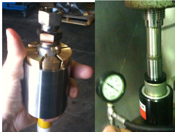
Figure 5: Testing the concept wedges to determine axial force required to obtain equivalent radial compression of fitting and to check for leaks.
