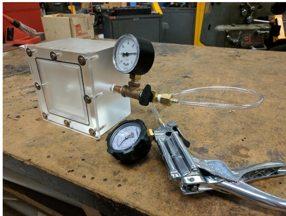
Figure 4.3. The realized Acoustic Energy Harvester design.
